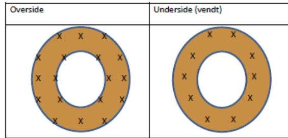
Figure 5. Sampling of homogenized sample
